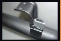
O.E. style heavy duty hangers and brackets connect to all orginal mounting points on vehicle.
